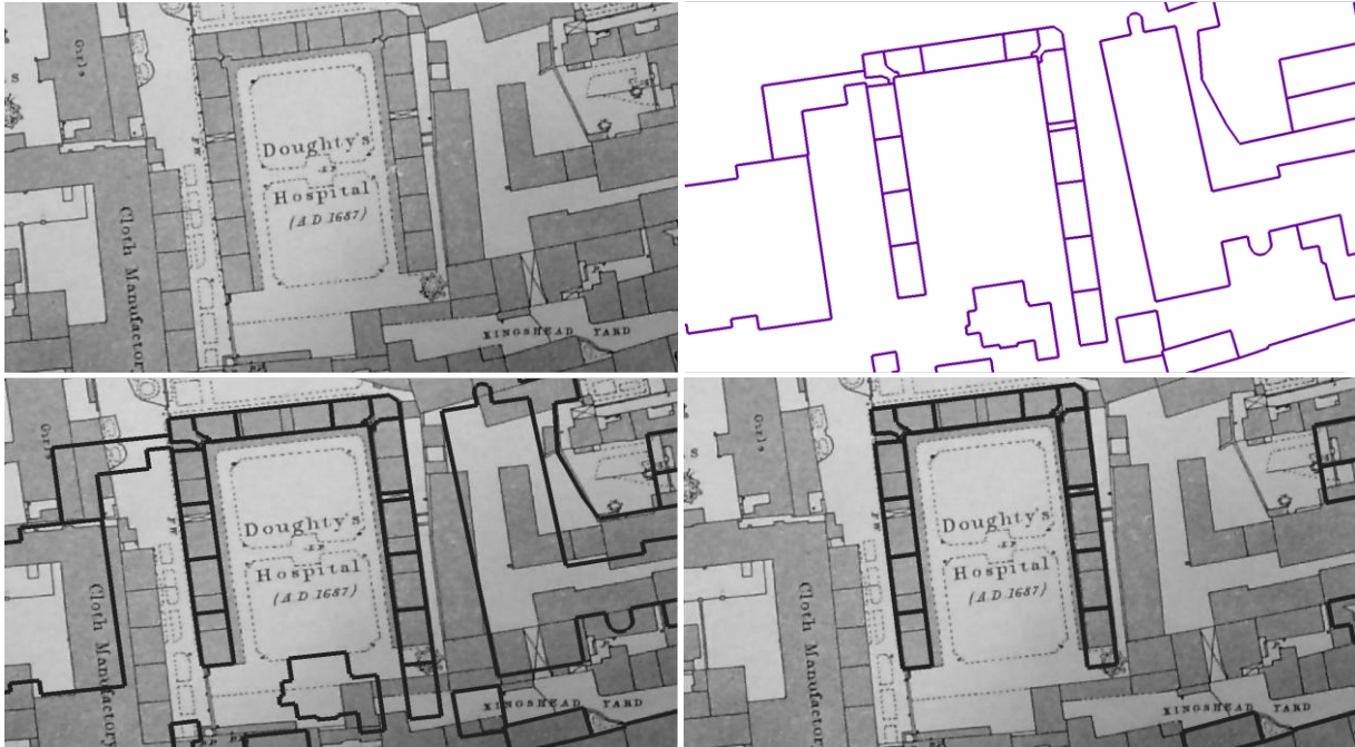
Figure 6 Added feature to the Footprint Extractor for aligning maps and vector data to a historical map; (top right) input vector data; (bottom left) Alignment result; (bottom right) Final result showing the preserved vector data after matching.
