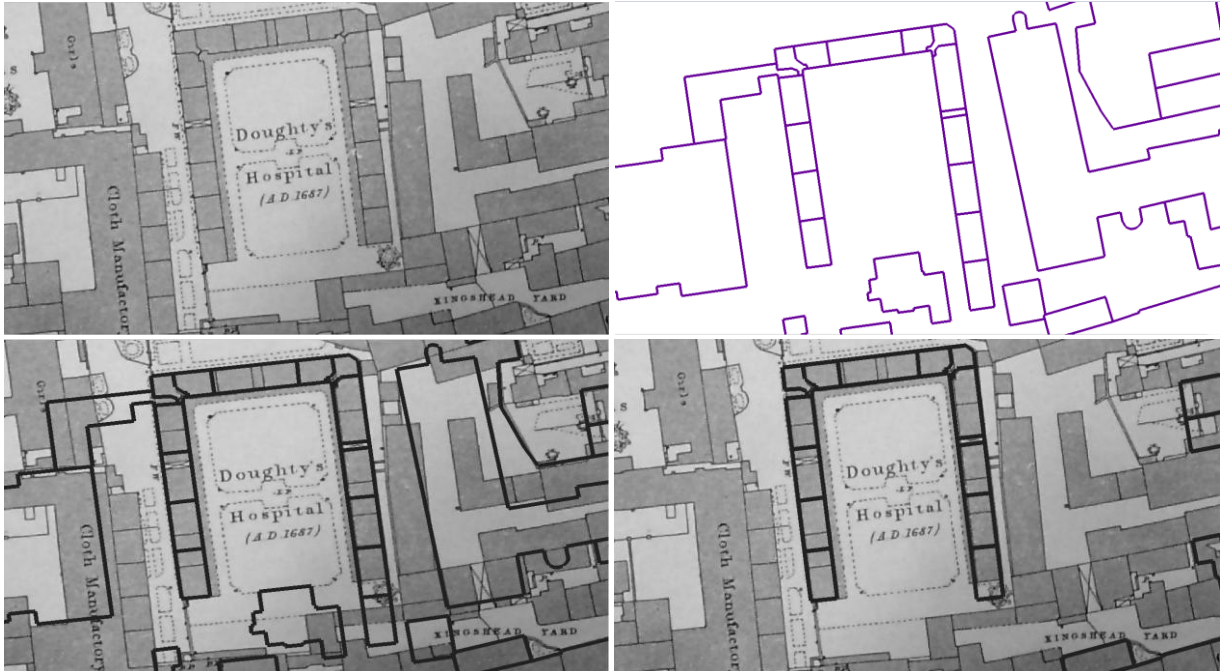
Figure 6 Added feature to the Footprint Extractor for aligning maps and vector data; (top left) historical map; (top right) input vector data; (bottom left) Alignment result; (bottom right) Final result showing the preserved vector data after matching.
