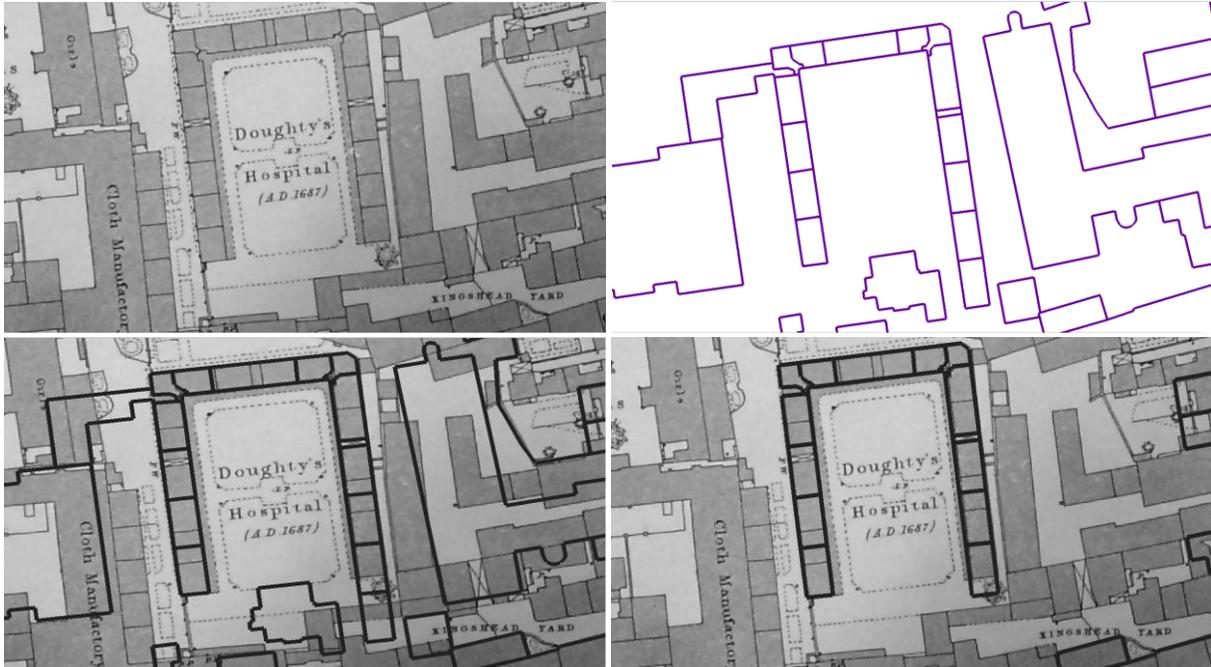
Figure 6: Added feature to the Footprint Extractor for aligning maps and (top left) historical map; (top right) input vector data; (bottom left) Alignment result; (bottom right) Final result showing the preserved vector data after matching.
